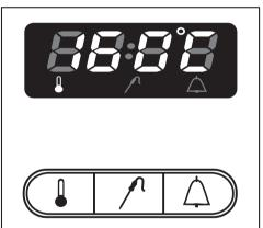
As soon as a heating system is selected, the **recommended temperature** for that system appears in the oven display and the oven heating comes on.
